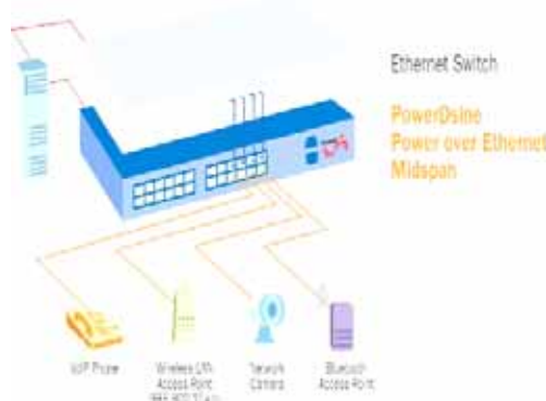
Figure 1: Brand new PoE-enabled switch vs. Midspan added to existing network switch
