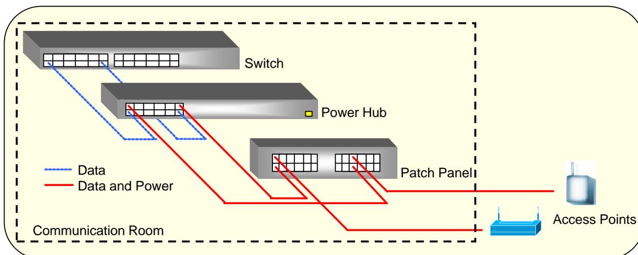
**Figure 2: Installing WLAN with Power over LAN**
